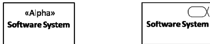
Figure 40 – Example visualizations of the Alpha meta-class construct and its Software System type
